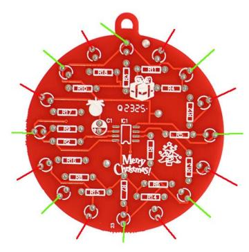
2. Solder the IC to it's place. Note that it have polarity and there is mark on the PCB and IC to follow.
