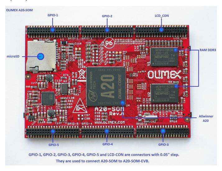
Please note that there might be differences in the layout of top of the board compared to the latest revision. One of the notable changes introduced in hardware revision C of the design, is the addition of GPIO-6 row of pinholes that provides easier access to some additional pins. The general routing and memory positions are also adjusted.
