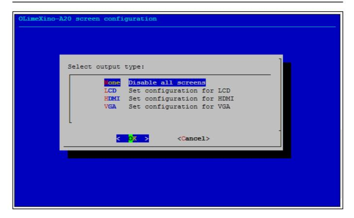
Choose the resolution and the interface (LCD, HDMI or VGA).
