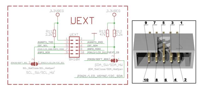
\*Note the two jumpers PIN29/SOFT\_CL – PIN22/LCD\_EN/I2C\_SCL, and PIN28/SOFT\_SDA3 – PIN21/LCD\_HSYNC/I2C\_SDA which by default are set to a software SPI. They can be used to set the whole UEXT to a hardware SPI.
