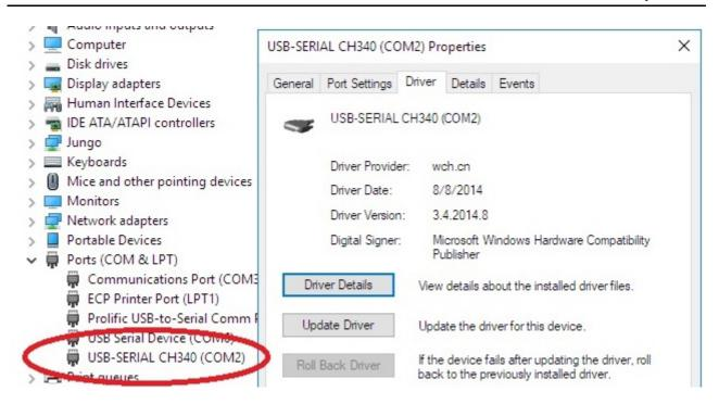
The serial cable that we use gets assigned COM #2. We need this information in order to start the PuTTY on the same serial port. Start your serial terminal software. PuTTy is shown below – select the proper COM port, the speed, make sure that the connection is set to "Serial" and finally click "Open" at the bottom:
