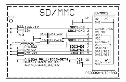
The SD/MMC2 slot is located on the back of the PCB and works with the "larger" SD and MMC cards. The connector was placed by a popular demand.
