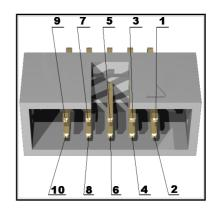
PIN0, PIN1, PIN2 and PIN3 are connected to the power regulator module AXP209.
