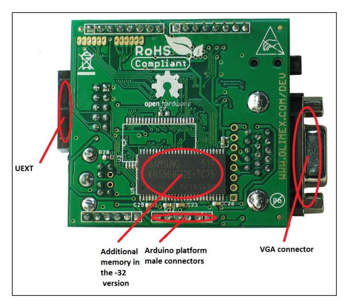
Note the base MOD-VGA version doesn't have the additional memory present on the picture of MOD-VGA-32.
