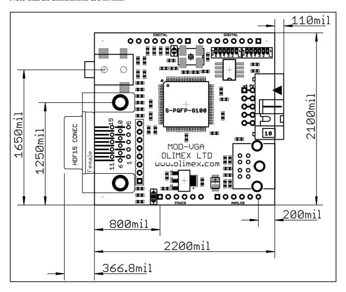
The two highest elements on the board are: VGA connector – 500mil; KEYBOARD connector – 500mil
