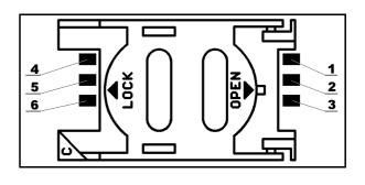
This is standard SIM card connector, to operate MOD-GSM should have inserted valid SIM card for your operator network.
