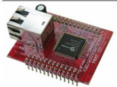
**DM9000E-H** is low cost 10/100 Mbit Ethernet controller development board based on DM9000EP with flexible options to be addressed with 8-16-32 bit data buses microcontrollers and support for MDI-X.
