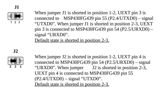
Depending on jumpers J1 and J2 configuration, the board can work in host, or in device mode. The default state of J1 and J2 is for device mode (shorted in position 2-3).
