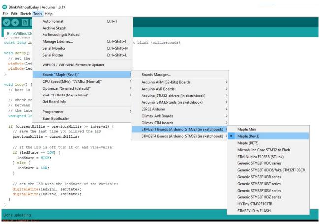
Select the port where the board is listed (remember to install drivers from archive if it is not listed) and load a demo. Here is a blink demo you can use as first demo:
