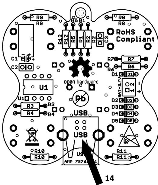
14. A USB type B connector at position **USB**. The connector is placed at the same side of the board as the microcontroller! Double check for short-circuits between the pins before powering!
