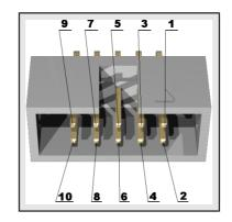
IMPORTANT: Be careful with the voltage levels of the signals of the UEXT and specifically the output available at pin #1. The on-board 3.3V/5V switch also controls the voltage output of the UEXT! Do not connect Olimex modules when the switch is set to 5V position, unless you are 100% sure that these UEXT modules work fine at 5V (most Olimex modules can not work properly at 5V, only at 3.3V)
