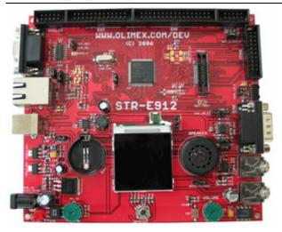
STR-E912 is low cost development board for the new STR912 ARM966E-S microcontroller from ST Microelectronics. With 512KB internal flash, 96KB internal RAM, USB, CAN, RS232, 10/100 Ethernet, SD/MMC card connector, Audio In/Out, TFT color LCD, joystick for menu navigation, connectors for the external memory bus, JTAG, TRACE this board allows all STR912 features to be explored. The demo codes show how easy can be build USB mouse, USB HID Audio device, open source web server, LCD interface.
