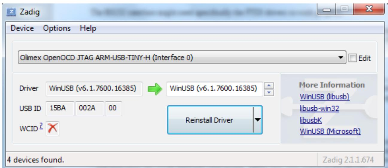
If Zadig doesn't do the job or you are using OpenOCD version prior to 0.8.0 the more robust method is to download an archive with the drivers and point the Windows Device Manager to it manually. Links to those resources might be found at the end of this chapter!
