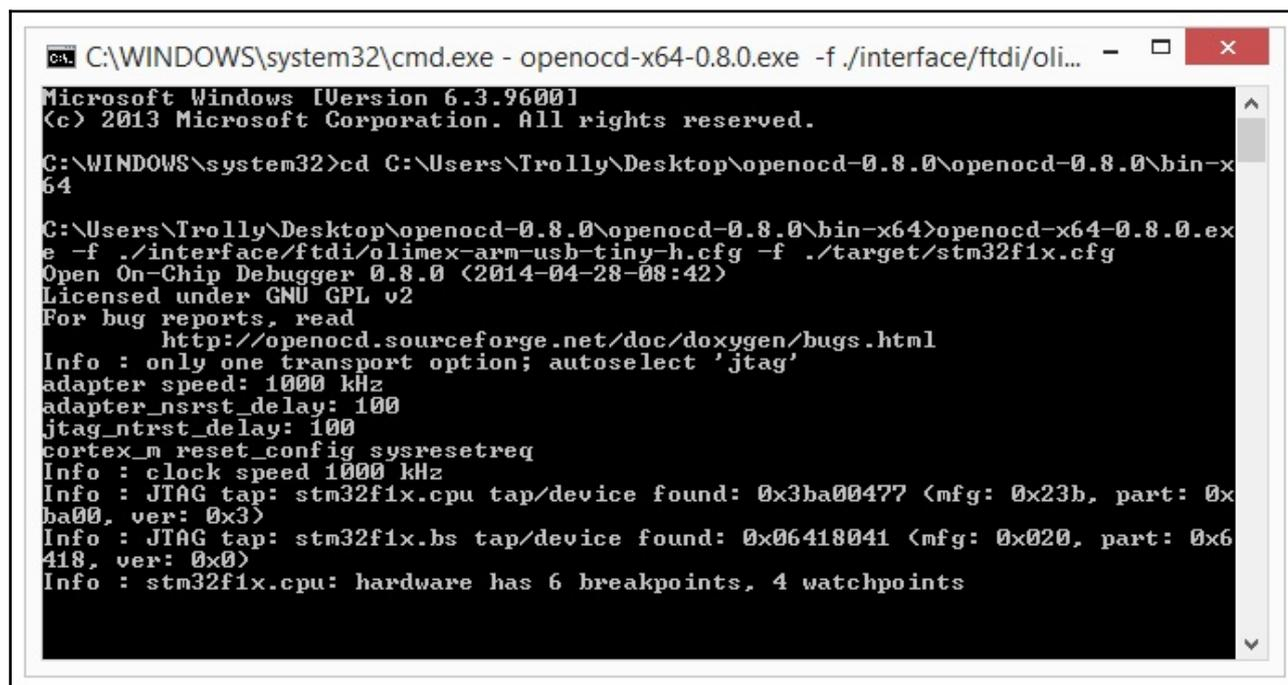
After establishing the GDB server connection described below you can open new terminal and run a telnet connection. The telnet would accept commands on port 4444. More info might be found here: [https://www.olimex.com/Products/ARM/JTAG/resources/Manual\\_TELNET.pdf](https://www.olimex.com/Products/ARM/JTAG/resources/Manual_TELNET.pdf)
