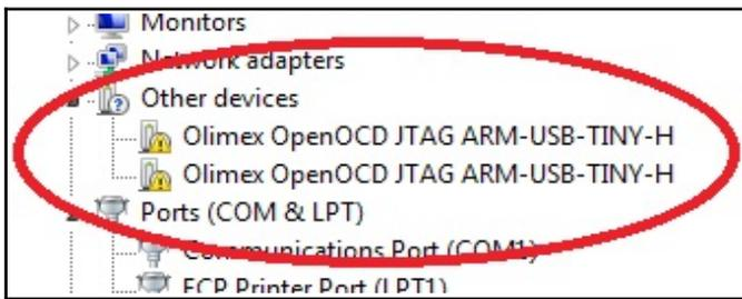
The driver installation in Windows would depend on which version of OpenOCD you are using. There is a difference in the driver installation if you are using OpenOCD 0.8.0 or newer and if you are using versions prior to OpenOCD 0.8.0.
