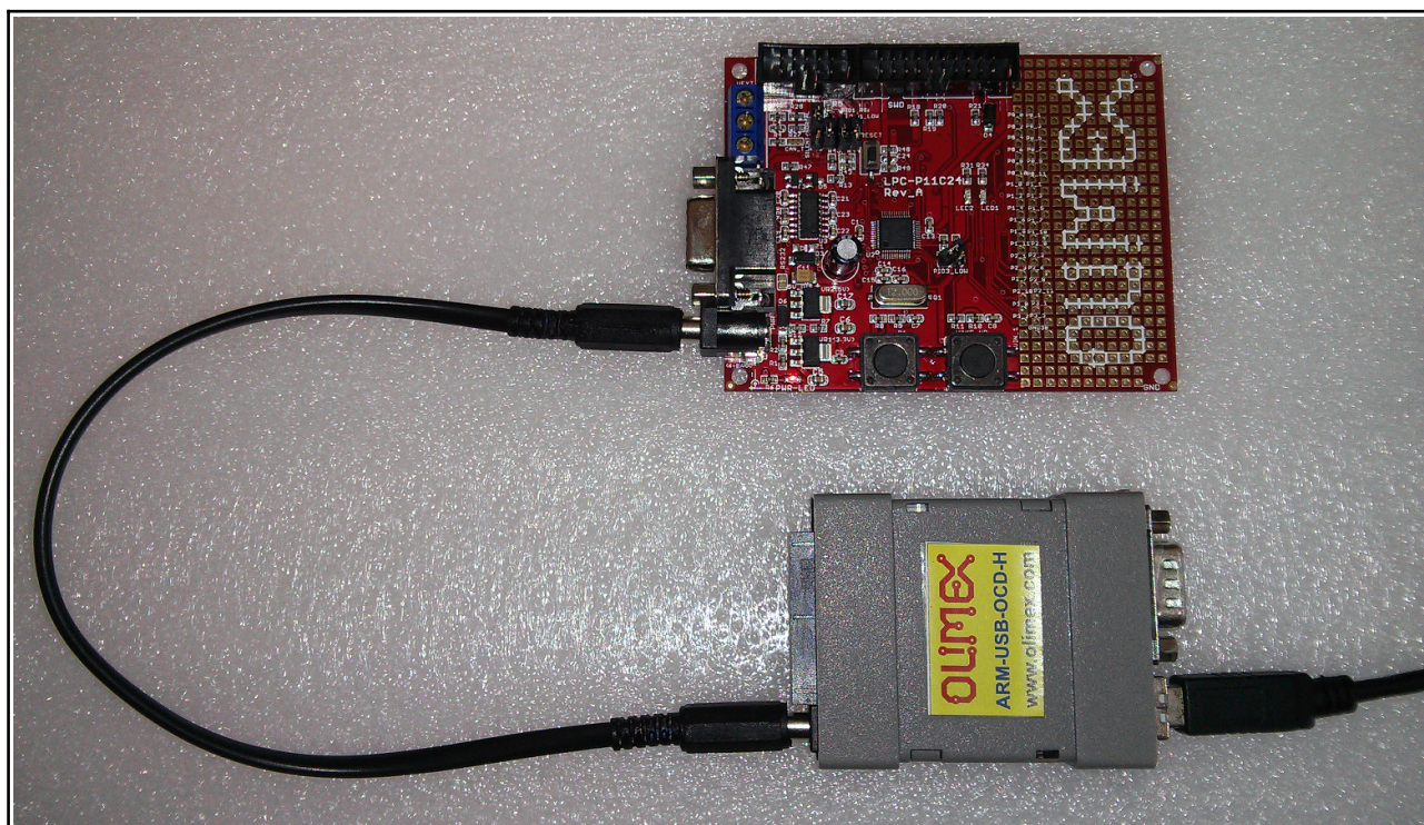
ARM-USB-OCD-H powering LPC-P11C24 (via the PWR_OUT jack).
