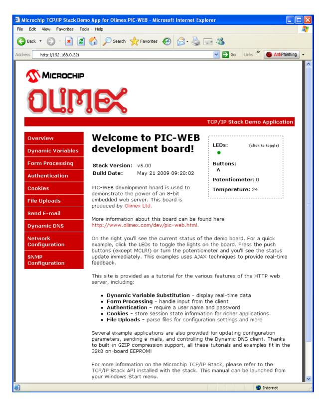
At the picture above, you can see the default page that you must get. It shows the temperature of the on-board thermistor, the status of the button BUT, the value of the potentiometer, the status of the LED and so on.
