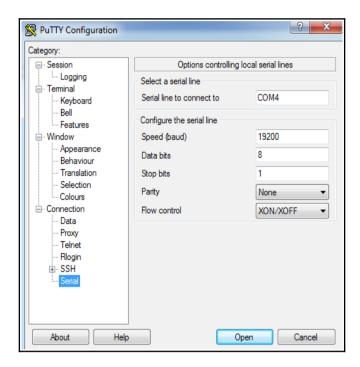
NOTE: The field "Serial line to connect to" should be with value depending on the com port where you have connected the board. You can check that on the device manager menu, category "Ports (COM & LPT)".
