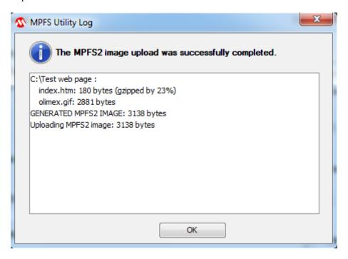
Please note that an image file (in this case MPFSImg.bin) is generated and may be used later if you select the 'Pre-built MPFS image' radio button at the top of the utility program window.
