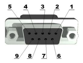
**TXD** Output **Transmit Data.** This is the asynchronous serial data output for the RS232 interface.
